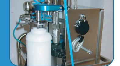
At the back of the device is a special filter holder. Here, all standard filters can be adapted directly on the device, from syringe filters to standard capsules.
