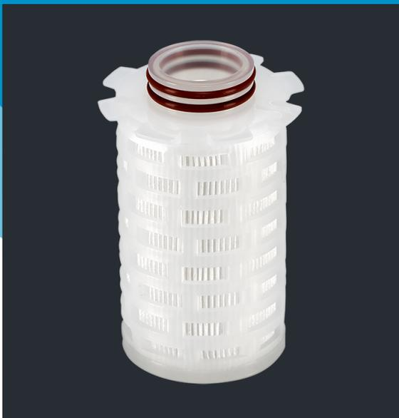
BorsoPTFE-JM junior cartridges are manufactured with a zPTFE membrane with a reduced resistance to flow while fully retaining bacteria. The cartridges are highly resistant to thermal stress during steam sterilization. A multitude of adaptor options are available for easy retrofitting into existing housings.
